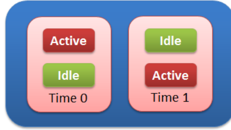
Figure 6.5: One core is active at each timestamp, resulting in an active package.
